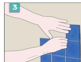
Press tile into properly placed setting material.
